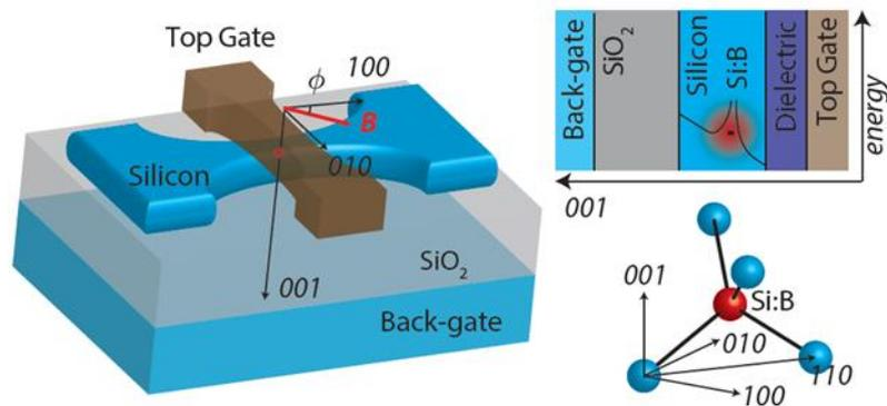
Fig. 1. Sketch of the device geometry and layered heterostructure in the (001) direction. The orientation of the magnetic field within the plane is given by  $\phi$ , the angle with respect to the (100) direction.
